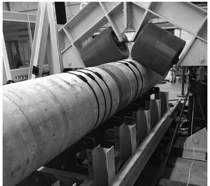
7.2.6] SP-500-1721 with Smart® Tie 20mm (¾") and Smart® Tie 32mm (1¼")
